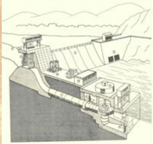
Figure 2-1 Typical Vermont Hydropower Installation. The walls of the powerhouse and intake structure are removed to illustrate the project works: (1) Dam with flashboards, (2) waste gate and gatehouse, (3) intake spill, (4) trash rack, (5) intake gate, (6) intake gate head, (7) penstock, (8) shut-off valve, (9) turbine, (10) draft tube, (11) generator, (12) switch gear, (13) transformer, (14) circuit breaker, (15) draft tube gate and head.
